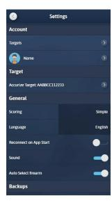
Accurize comes with three scoring systems and can be adjusted any time from the settings screen.
