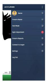
Using Auto Sight Adjustment mode you can adjust the current firearm / target's sight adjustment by firing at the target itself. When in sight adjustment mode the bottom bar is green.
